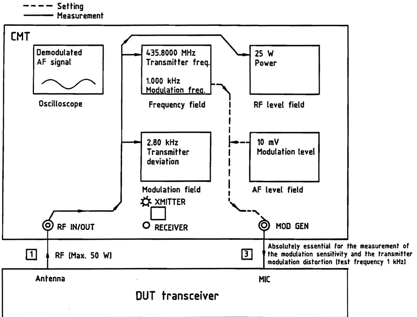
Fig. 2-11 Transmitter test
