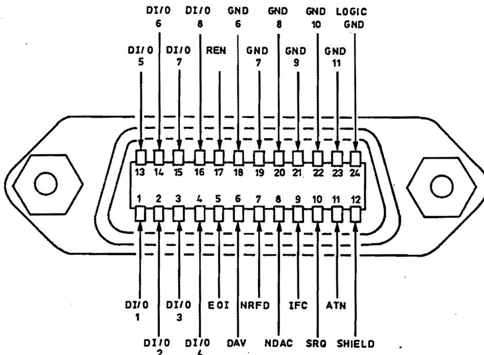
Fig. 2-14 Pin assignment of IEC-bus connector 103
