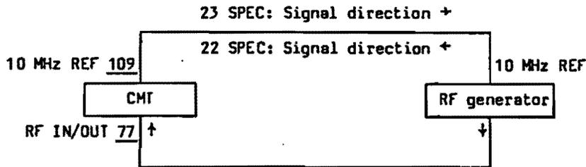
1. Apply unmodulated signals between 400 kHz and 1 GHz.
