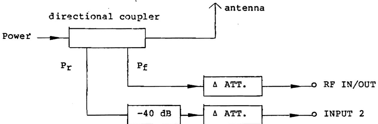
By inserting an additional 40-dB attenuator, the difference in sensitivity between both inputs is balanced.
