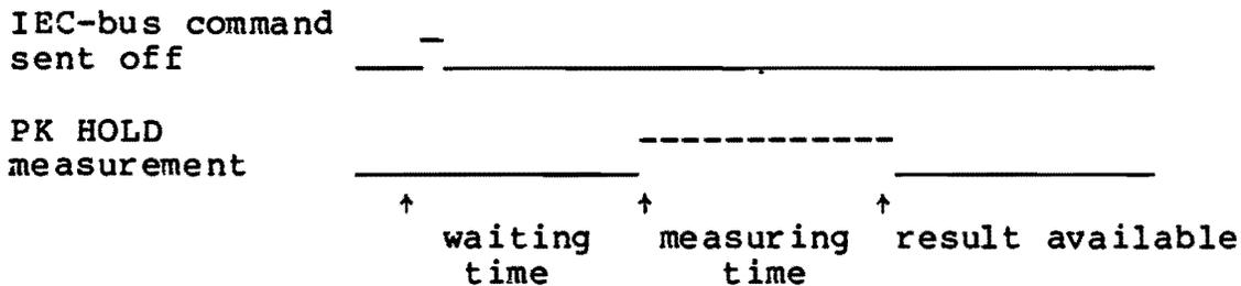
These times can be set between 0.1 and 3 s via the two functions
