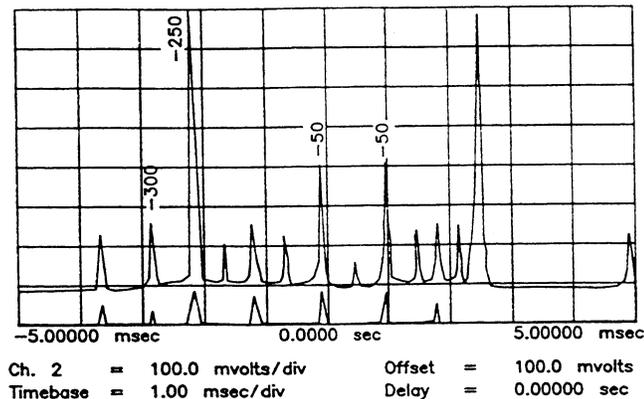
*Figure 5-18. Frequency Response of Notch Filters, 965 MHz Setting.*
