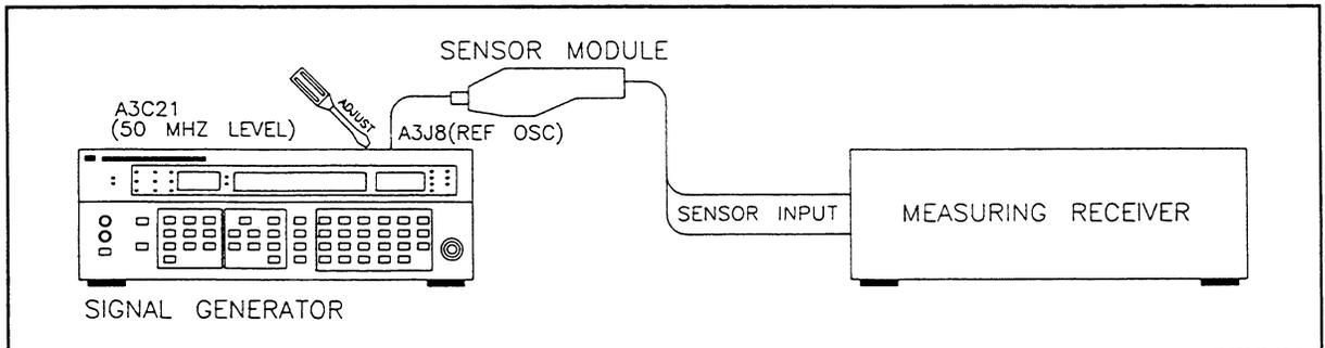
Figure 5-7. 50 MHz Reference Oscillator Level Adjustment Setup
