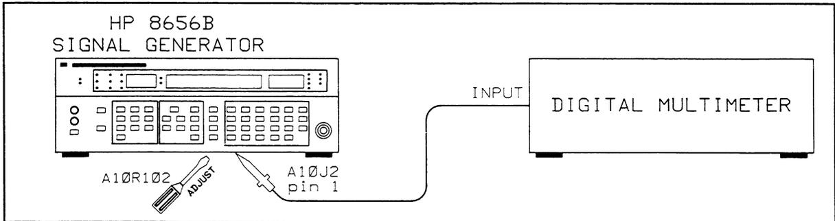
Figure 5-1. HP 8656B Power Supplies Adjustment Setup
