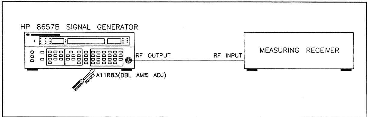
Figure 5-26. AM% and ALC Loop AM Adjustments Setup
