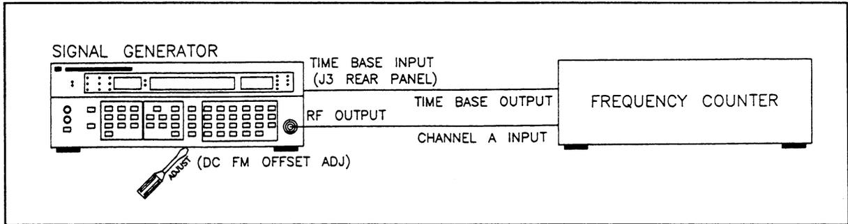
Figure 5-34. DC FM Frequency Offset Adjustment Setup
