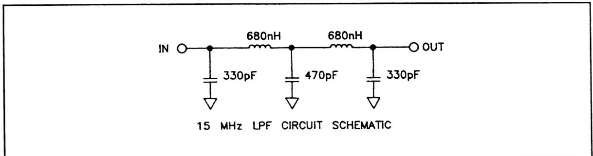
*Figure 4-15. Schematic for 15 MHz Low Pass Filters*
