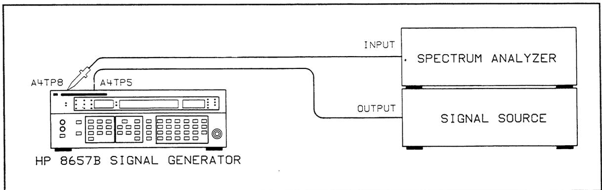
*Figure 5–15. HP 8656B Notch Filters Adjustment Setup*
