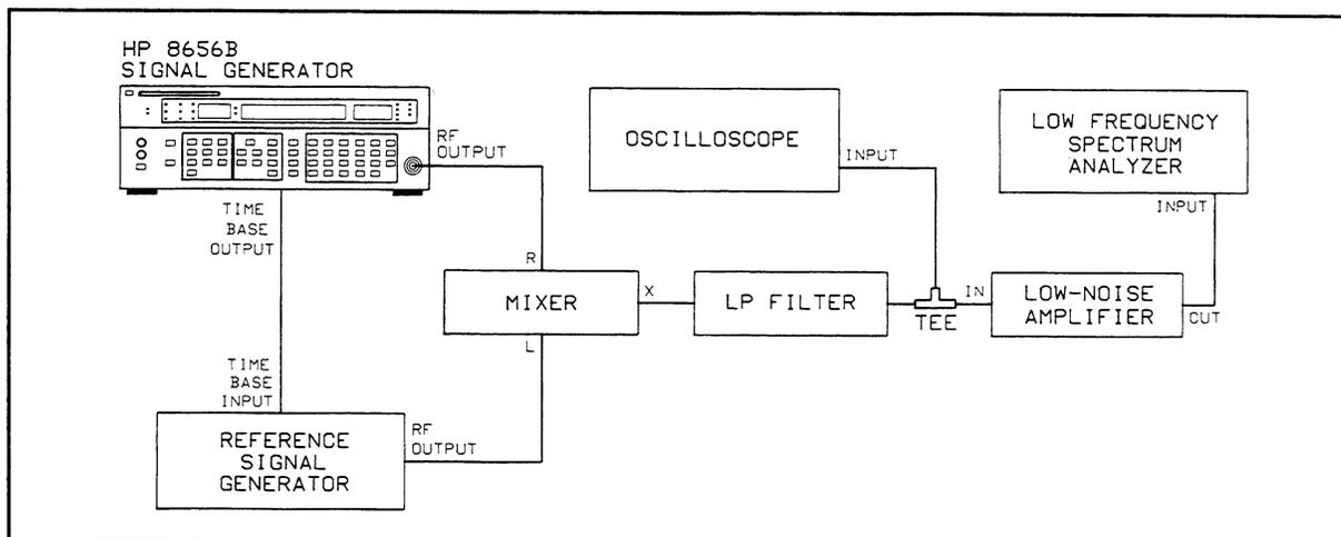
**Figure 4-6.** HP 8656B SSB Phase Noise Measurement Set-up
