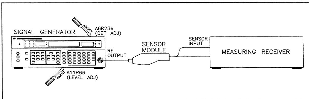
Figure 5-24. Level and ALC Loop Detector Adjustment Setup
