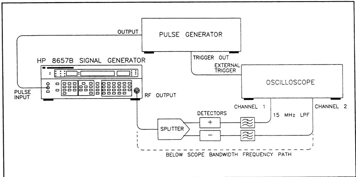
*Figure 4-14. Rise/Fall Time Test Setup with Peak Detectors*
