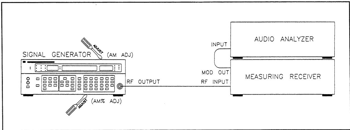
*Figure 5-25. AM% and ALC Loop AM Adjustments Setup*
