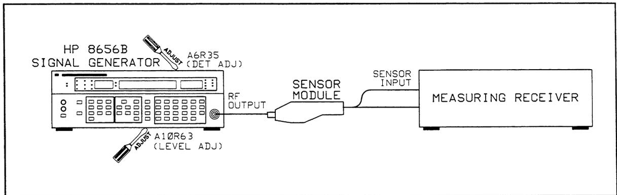
Figure 5–21. Level and ALC Loop Detector Adjustment Setup
