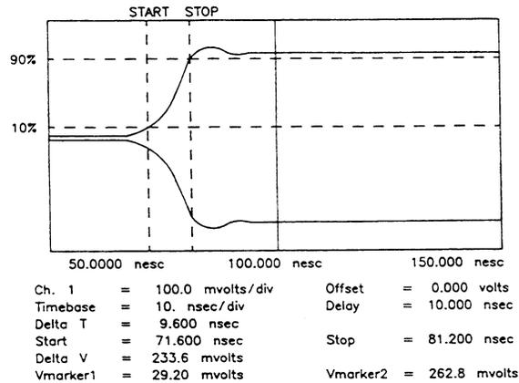
*Figure 4-13. Oscilloscope Display*
