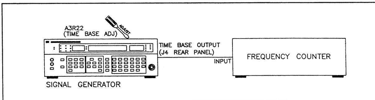
*Figure 5–8. 50 MHz Reference Oscillator Frequency Adjustment Setup*
