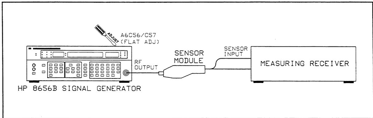
Figure 5–23. Heterodyne Band Accuracy and Flatness Setup
