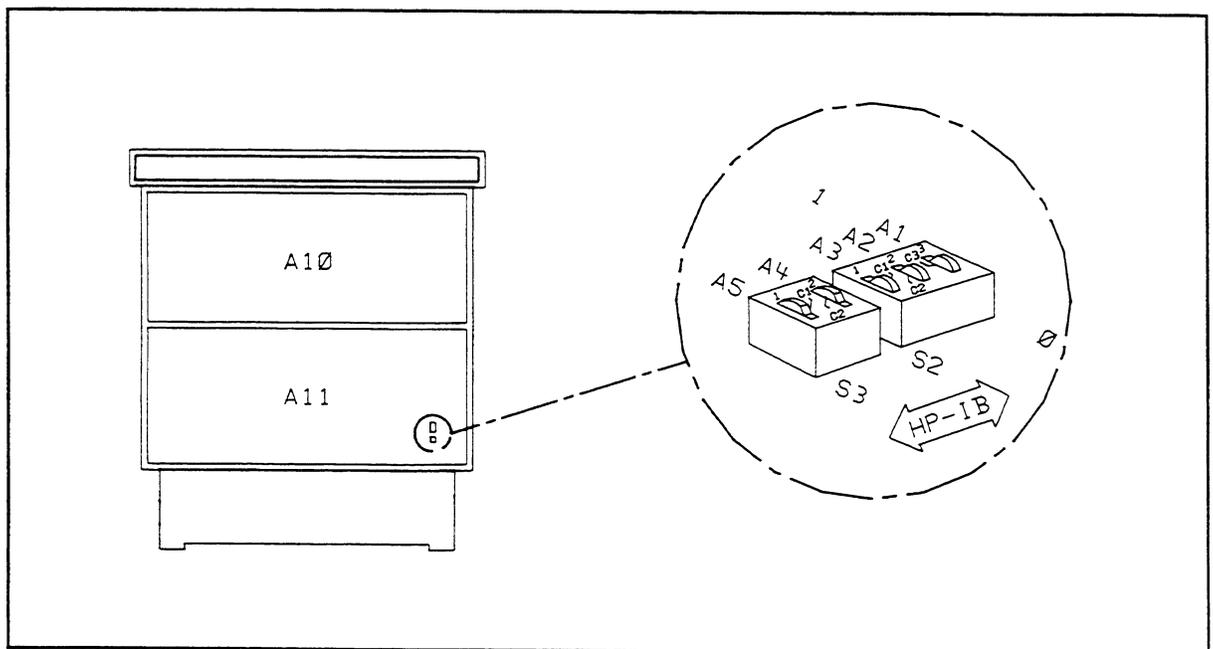
*Figure 2-3. HP 8656B/8657A HP-IB Address Switch Location and Settings*
