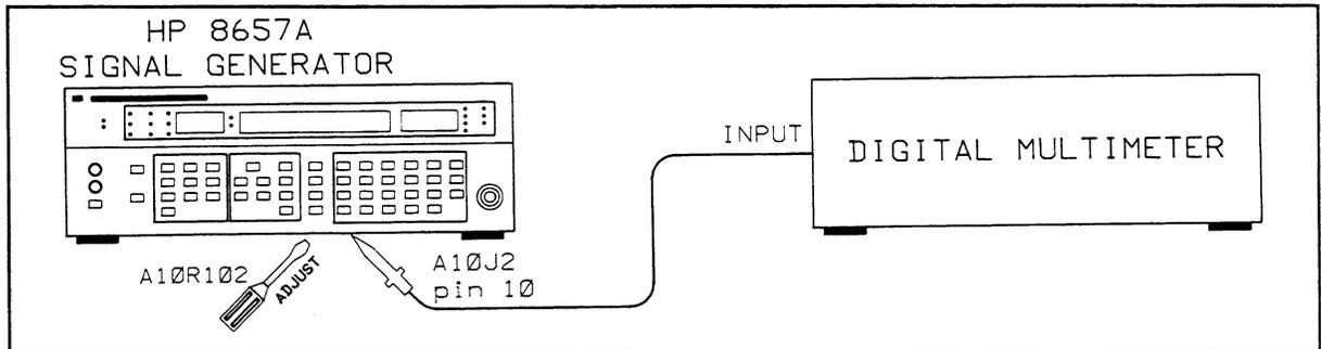
Figure 5-2. HP 8657A Power Supplies Adjustment Setup
