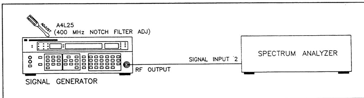
Figure 5-20. 400 MHz Notch Filter Adjustment Setup.
