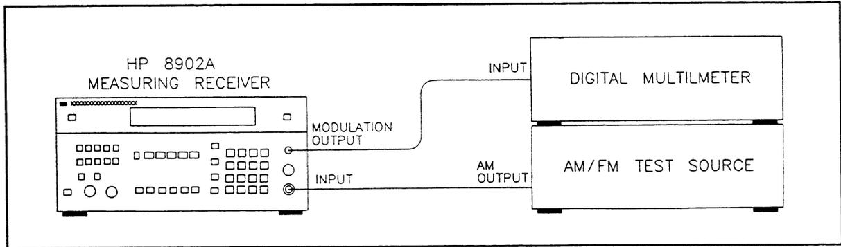
Figure 4–2. Measuring Receiver Residual AM Verification Test Setup
