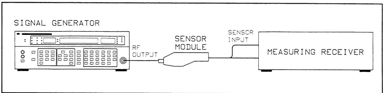
*Figure 4-8. Output Level Accuracy and Flatness Test Setup*
