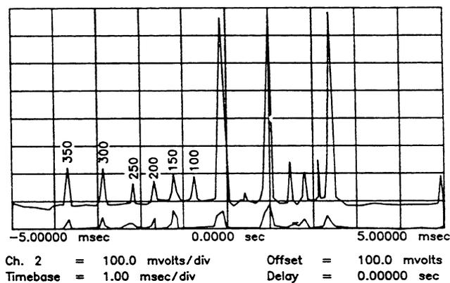
*Figure 5-17. Frequency Response of Notch Filters, 765 MHz Setting.*
