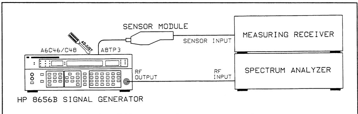
*Figure 5-22. Heterodyne Band 800 MHz Bandpass Filter Adjustment Setup*
