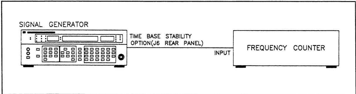
*Figure 5-37. 10 MHz Reference Oscillator Frequency Adjustment Setup*
