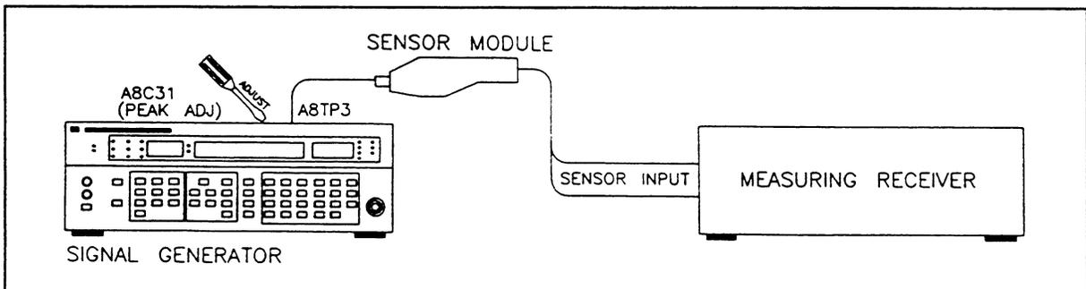
Figure 5-10. 400 MHz Bandpass Filter Adjustment Setup
