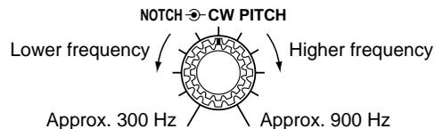
34 **MANUAL NOTCH FILTER CONTROL [NOTCH]** (inner control; p. 27)
