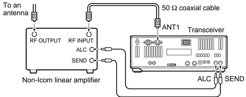
The specifications for the SEND relay are 16 V DC 2 A. If this level is exceeded, a large external relay must be used.
