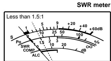
▨ The built-in antenna tuner matches the transmitter to the antenna when the SWR is lower than 3:1.
