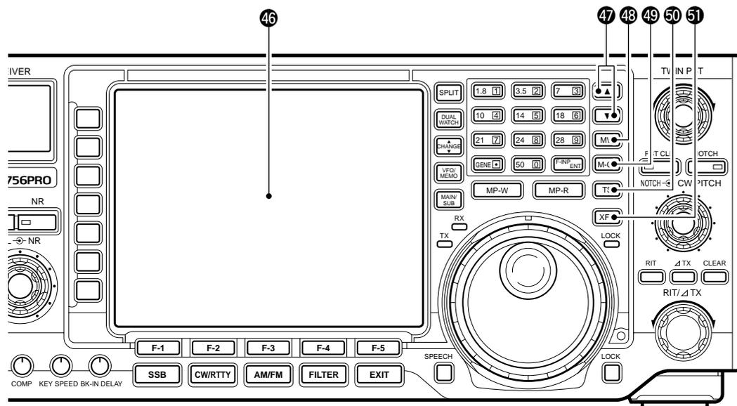
**46 LCD FUNCTION DISPLAY** (See p. 10 for details.) Shows the operating frequency, function switch menus, spectrum screen, memory channel screen, set mode settings, etc.
