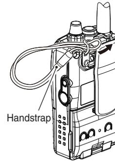
Slide the hand strap through the loop on the top of the belt clip as illustrated at left to facilitate carrying the transceiver.
