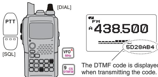
The DTMF code is displayed here when transmitting the code.
