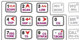
Depending on the tuning step setting, it may not be possible to input a 1 kHz digit. In this case, enter "0" as 1 kHz digit, then rotate [DIAL] to set the desired frequency.
