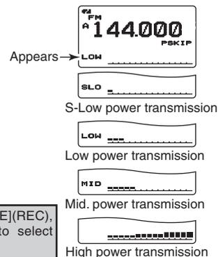
**WARNING! NEVER** continuously transmit for long periods of time. When the transceiver is used for continuous prolonged transmission at high power, the transceiver radiates heat to protect itself from overheating and transceiver's chassis will become hot. This may cause a burn.
