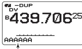
The received call sign is displayed while pushing and holding **[CALL/RX→CS]** when **[DIAL]** is rotated while **[CALL/RX→CS]** is pushed.
