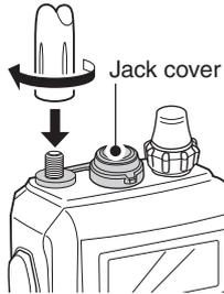
Insert the supplied antenna into the antenna connector and screw down the antenna as shown at left.
