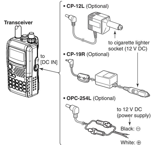
**NOTE:** Up to 5 W (approx.) of maximum output power is available when using external DC power. However, when the supplied voltage exceeds 14 V, the built-in protection circuit activates to reduce the transmit output power to 2.5 W (approx.).
