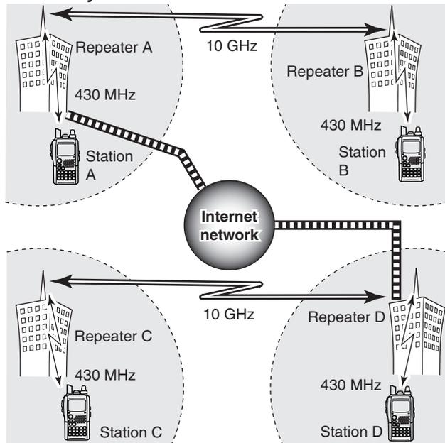
For current repeater operation, stations that are communicating must both be in the same repeater's operating area. However, in the D-STAR system as in the illustration at left, the repeaters can be linked via the system repeaters (with a 10 GHz signal). Thus stations A and B can communicate even though they are in different repeater operating areas.
