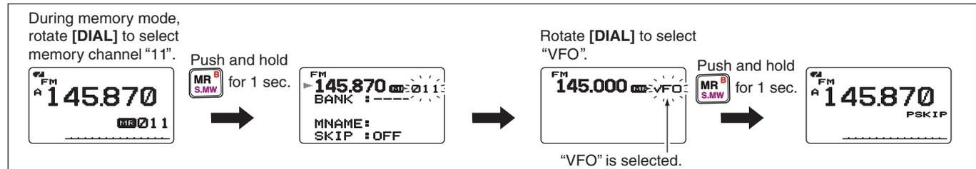
/// Holding **[S.MW](MR)** for 2 sec. at the step ②, will also copy the memory contents to VFO. In this case, the steps ③ and ④ are not necessary.
