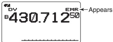
**NOTE:** The EMR communication function is turned OFF automatically when turning transceiver's power OFF
