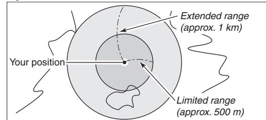
When the target position is coming into either/each area as above, the GPS alarm will sound.
