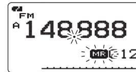
**Band memory scan function:** Repeatedly scans all memory channels programmed with any frequencies of the band programmed in the memory channel selected for scanning.
