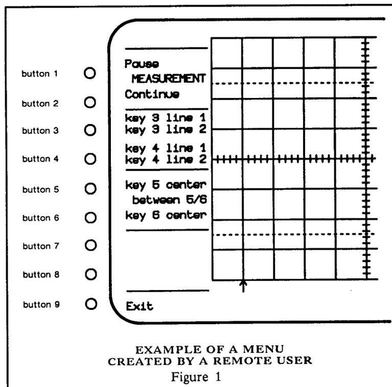
Text assigned to the menu buttons will disappear on the next transition to local but reappear when the instrument is switched back into the remote state. Text is cleared at power up, when the rear-
