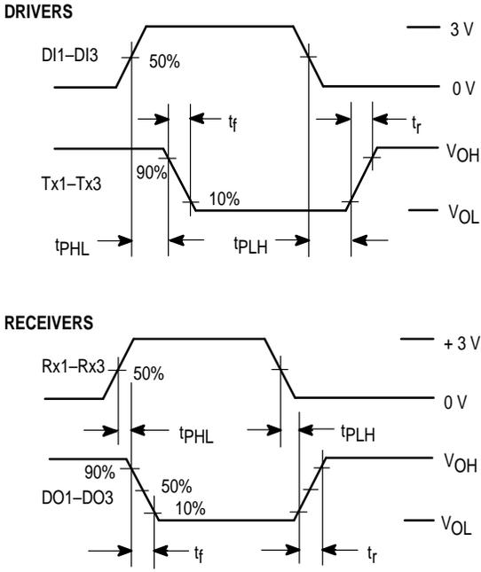
**Figure 2. Switching Characteristics**
