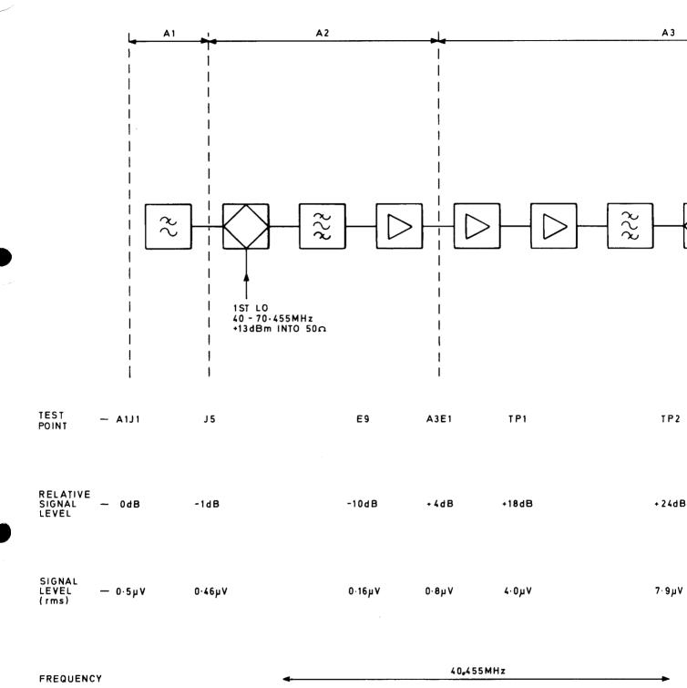
ALL SIGNAL LEVELS ARE RELATIVE TO ANTENNA INPUT AND ARE MEASURED USING AN RF OR AF VOLTMETER WITH HIGH IMPEDANCE PROBE. MEASUREMENTS MADE WITH AGC OFF AND IF GAIN SET TO MAXIMUM.
