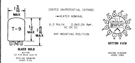
THE 6C10 CONTAINS THREE HIGH-MU TRIODES WITH SEPARATE PIN CONNECTIONS FOR ALL THREE CATHODES, GRIDS AND PLATES IN A COMPACT T-9 GLASS ENVELOPE WITH THE NOVEL 12 PIN BASE.
