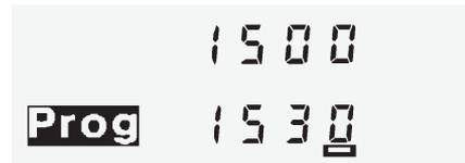
When the Fall Asleep Time is stored, the transceiver will return to normal operation.
