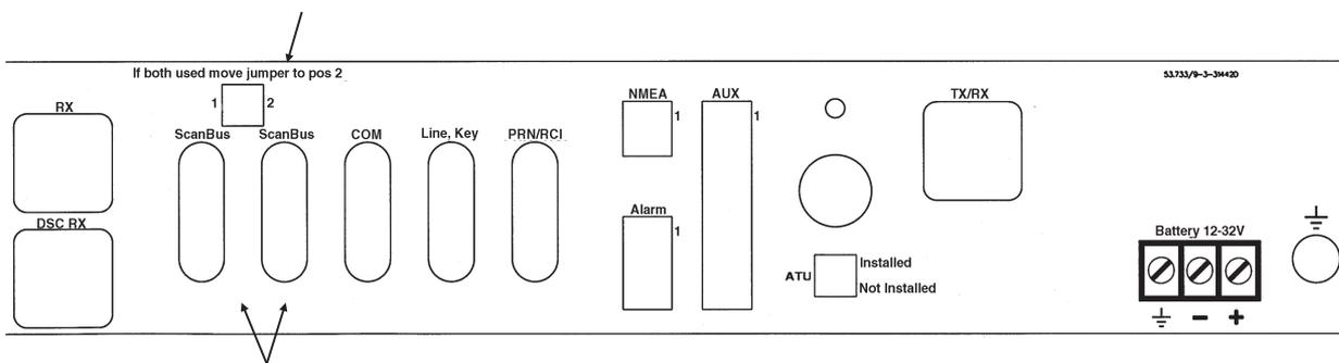
The ScanBus termination jumper must be set to pos. 1 if just one of the ScanBus connectors are used - and to pos. 2 if both ScanBus are used.
