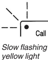
A call other than distress has been received. The lamp remains flashing until the call has been read out.
