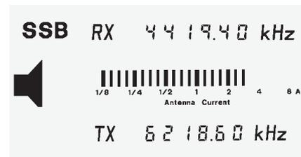
After the ATU tuning the bar-graph will display the RF current in the dummy load.
