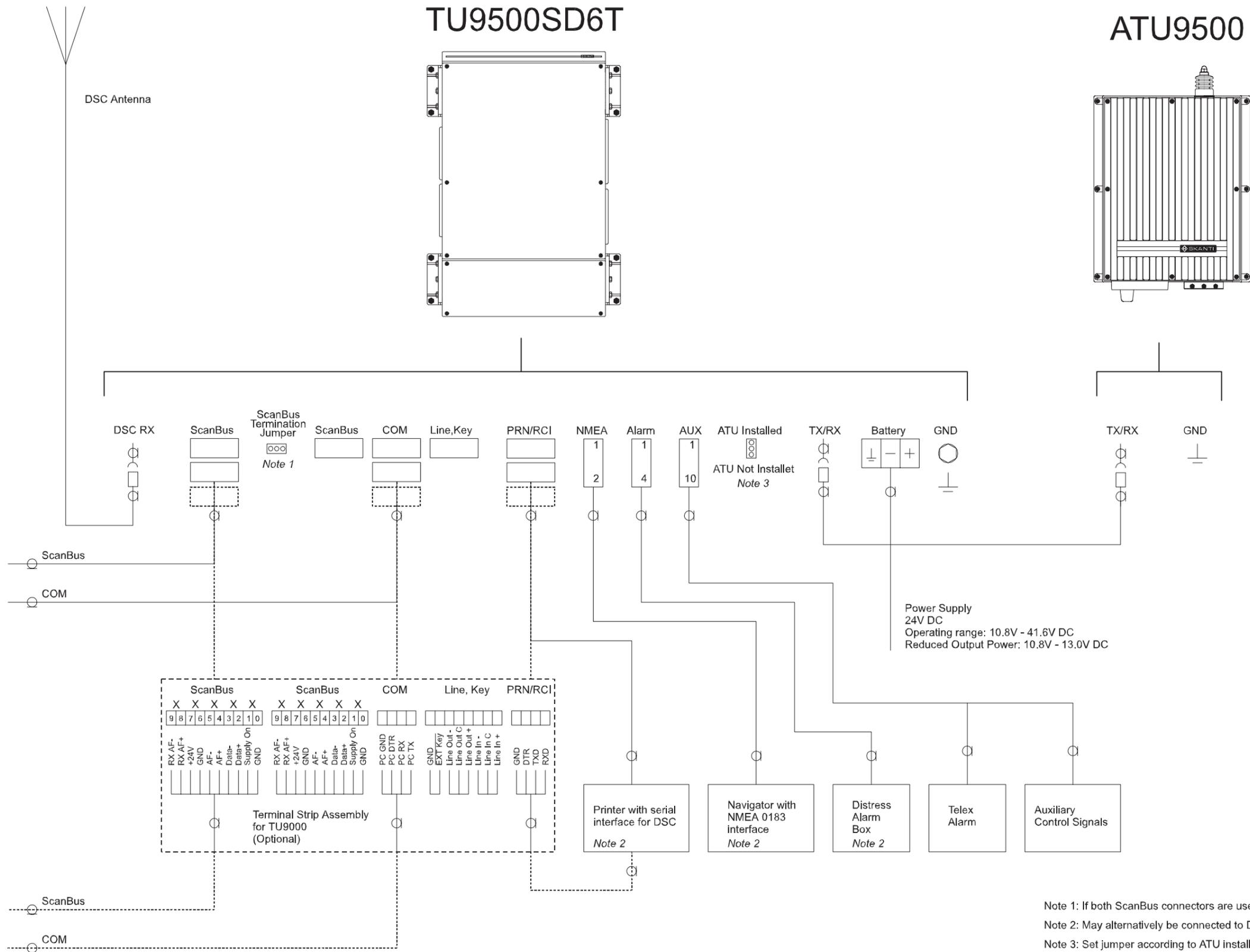
Note 1: If both ScanBus connectors are used move jumper to position 2.
