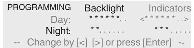
Select the "Night" setting for the display backlight using the arrow keys.
