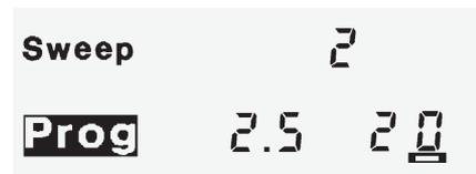
6. Enter the Step Frequency which is the frequency distance between all frequencies in the sweep.
