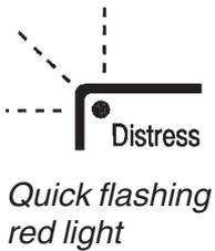
A distress alert will be transmitted if the Distress key is kept pressed for 5 seconds.
