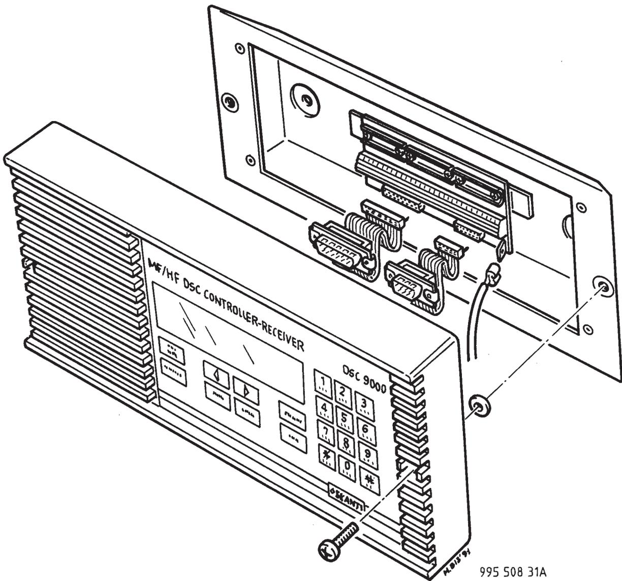
**DCU 9000 INSTALLATION WITH MOUNTING BRACKET**
