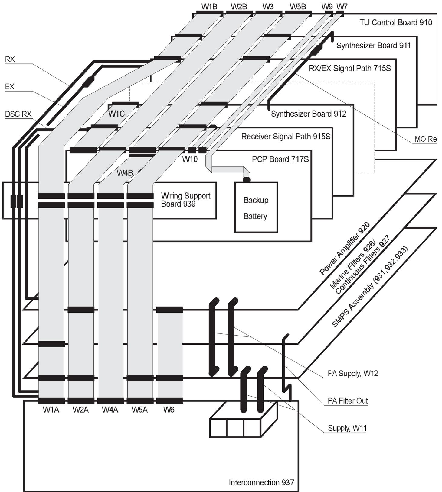
Local coax connections between Synthesizers and Receivers / Exciters are not shown.
