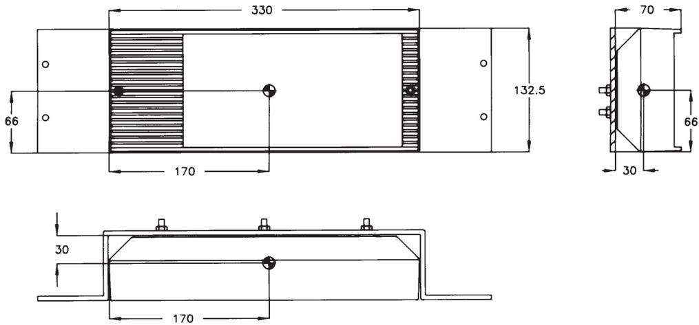
Dimensions are in mm Weight: DCU 1.2 Kg
