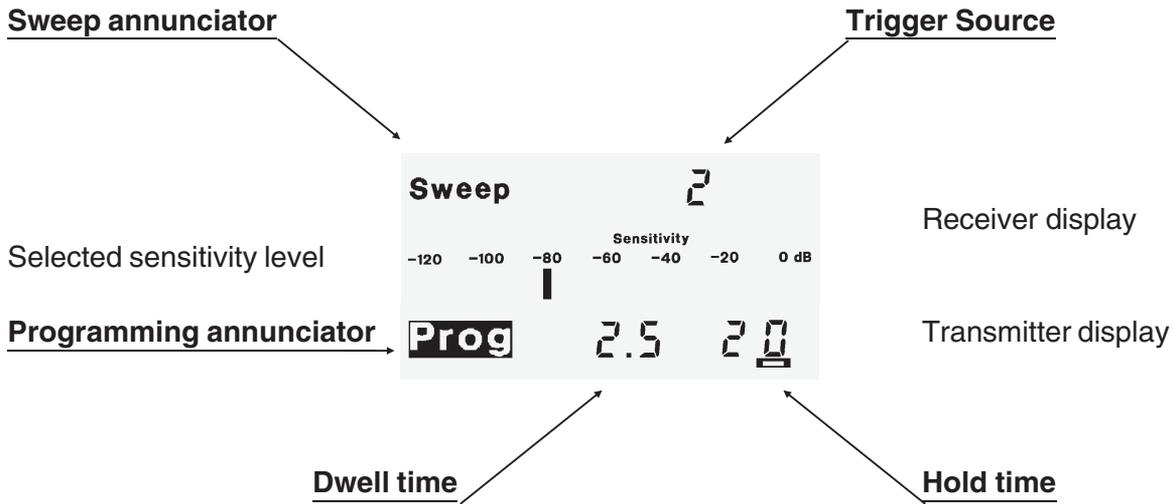
**Sweep annunciator** : Will be on during the programming and will flash during a frequency Sweep.
