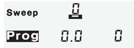
2. Enter the number of the Trigger Source that you want to use: 0 = no trigger source, 1 = squelch, 2 = signal strength, 3 = squelch or signal strength, 4 = squelch and signal strength.
