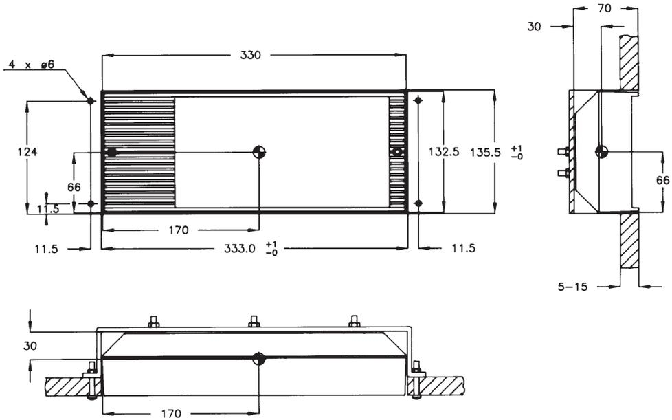
Dimensions are in mm Weight: DCU 1.2 Kg
