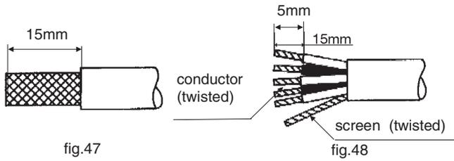
Before contacts of plug are soldered: slide the plastic cover over the cable.
