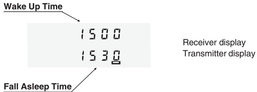
**Wake Up Time:** At this time the Sleep Program will switch on the transceiver.
