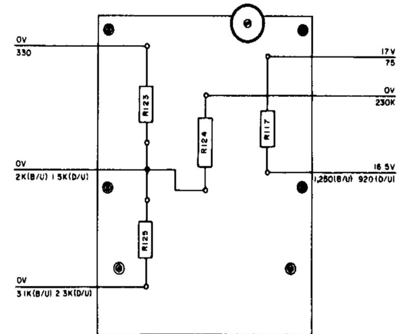
F RESISTOR MOUNTING BOARD TV-7B/U AND TV-7D/U
