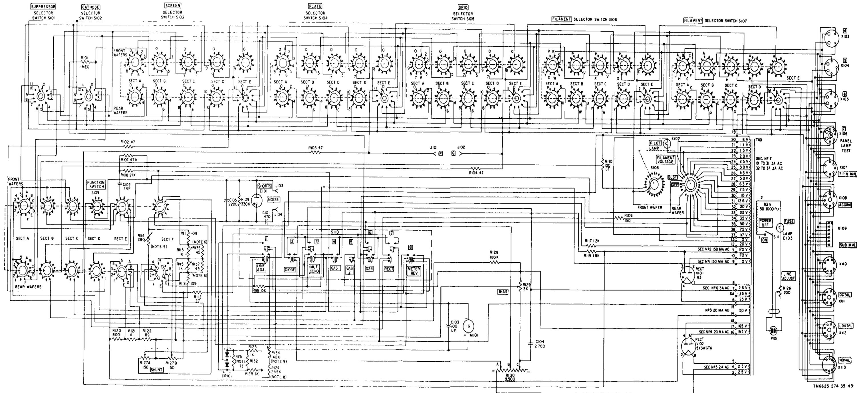
Figure 43. Test Sets, Electron Tube TV-A/U (serial numbers 1201 through 9492) and TV-7B/U, schematic diagram.
