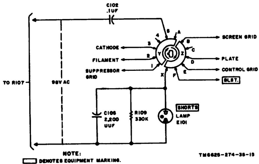
Figure 14. Simplified shorts test switch diagram.
