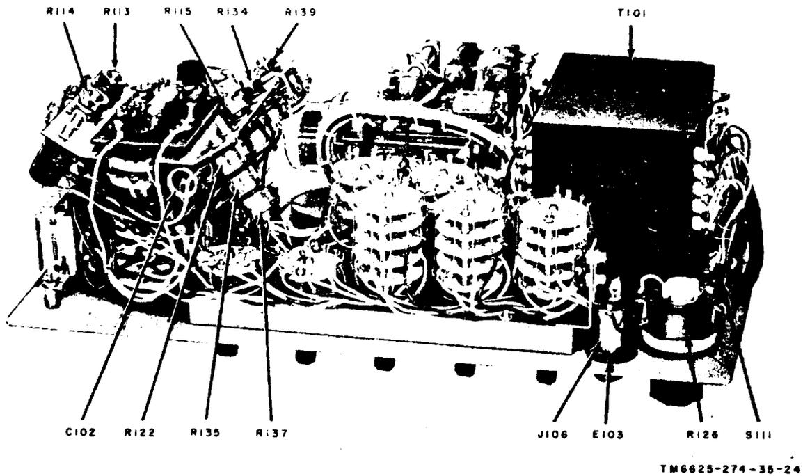
Figure 23. Test Set, Electron Tube TV-7DIU, front-right oblique.
